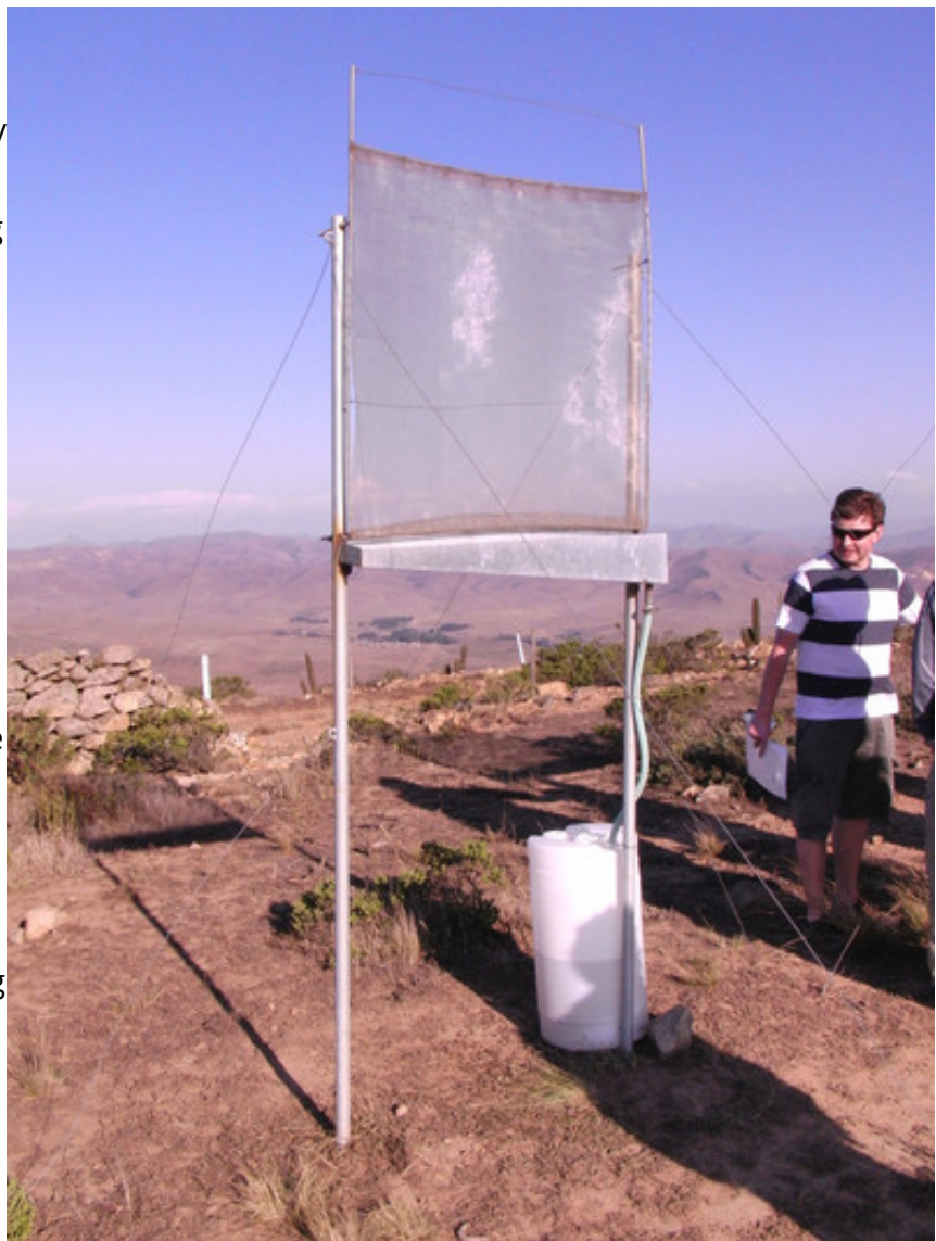
Water gets collected from a fog harvesting structure.
